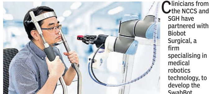
THE SELF-ADMINISTERED ROBOT, THAT AUTOMATES THE TAKING OF COVID-19 SWAB TESTS, WILL HELP REDUCE HEALTHCARE WORKERS' RISK OF EXPOSURE TO THE CORONAVIRUS
