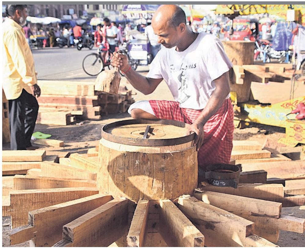
A Maharana servitor fixing an iron ring around the hub of a chariot wheel ahead of the Rath Yatra in Puri OP PHOTO
