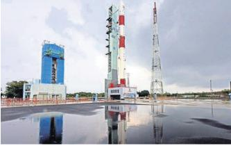
horse of ISRO -- can take up to 1,750 kg payload into SSO of 600 km altitude, according to ISRO officials. With lower per kg launch cost, the mini launcher will have
