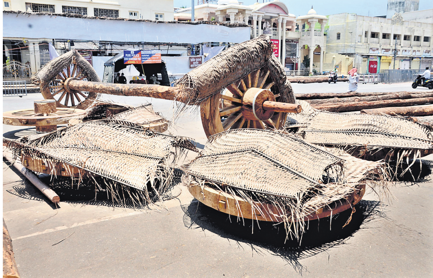
Newly-built chariot wheels covered with coconut leaf mats at Rath Yard in Puri to prevent cracks due to the scorching sun, Saturday
