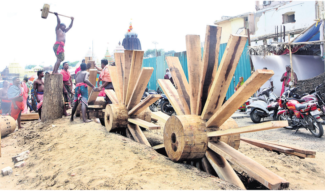
AT LORD'S SERVICE: Bhoi servitors attach spokes to hubs for chariots at Rath Yard in Puri, Friday
