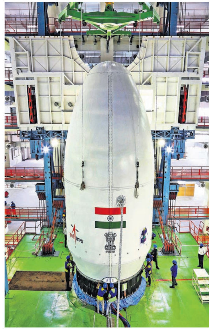
SPACE RACE: Chandrayaan-3 spacecraft being mated with LVM3 ahead of its launch, at the Satish Dhawan Space Station, in Sriharikota, Wednesday PTI PHOTO
