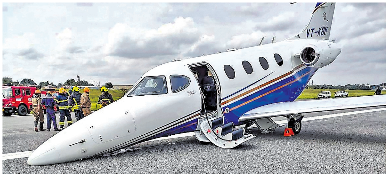
A private aircraft after it made an emergency landing due to a technical snag with its nose landing gear, at Hindustan Aeronautics Limited (HAL) airport in Bangalore, Karnataka
