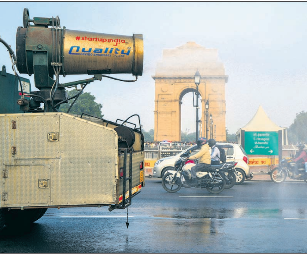
An anti-smog gun sprays water droplets to curb air pollution at India Gate, in New Delhi
