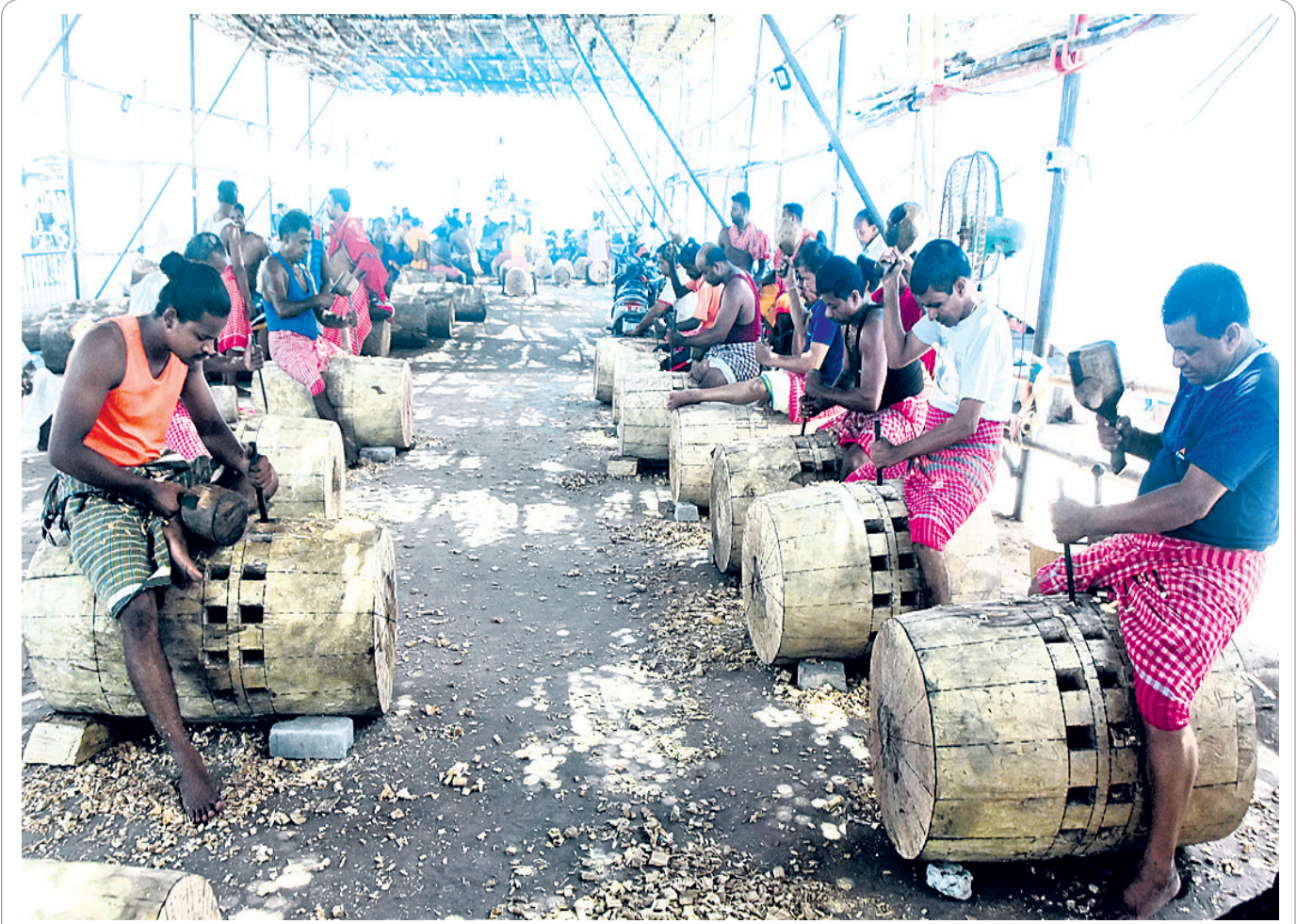
CAR FEST AHEAD: Maharana servants busy constructing hubs of chariot wheels at Rath Yard in Puri, Friday
